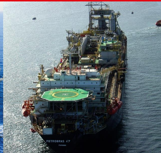
(FPSO) P-47 , 2005 Conversion of Floating, Storage & Offloading (FSO) P-47 into Floating Production, Storage and Offloading (FPSO) P-47, for the installation of an oil and water treatment unit to export treated oil from the Marlim to the Campos Basin.
