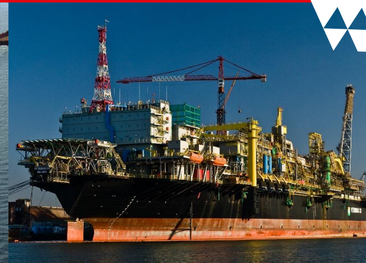
FPU P-53 , 2008 Supply of 8 modules, flare, pipe rack topsides for the FPU P-53, in Rio Grande-RS, (Related Company).
